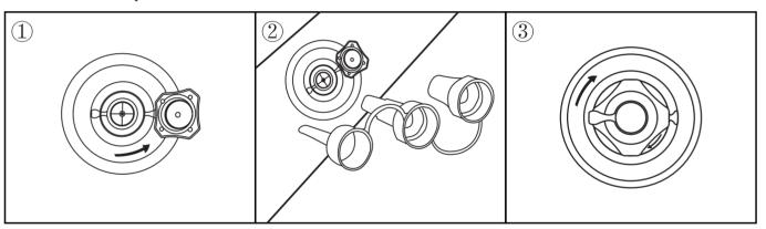
Unscrew the cap on the Inflation Valve for inflation.
